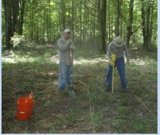
Intrusive investigation of subsurface anomalies identified during DGM survey.
