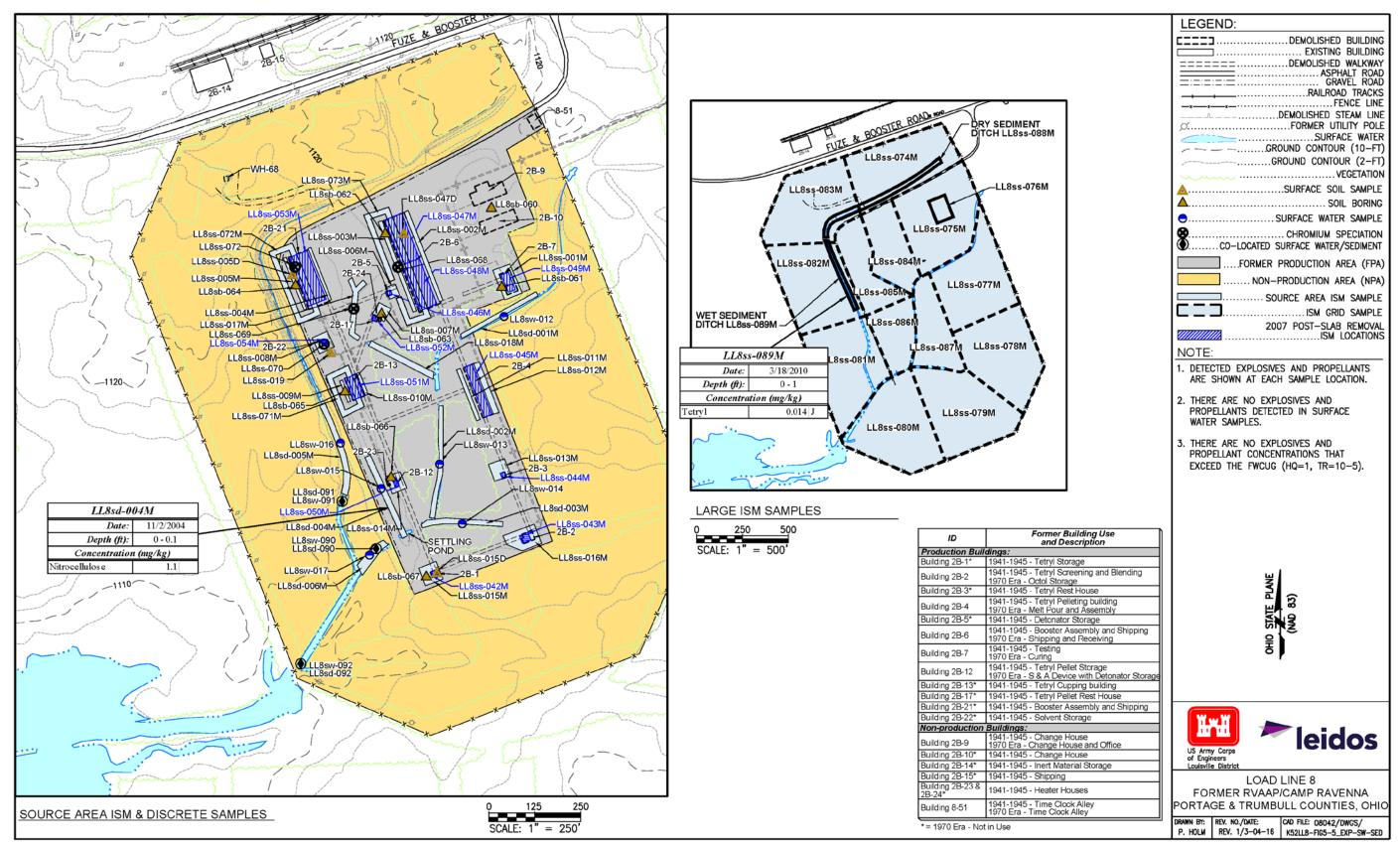
Figure 5-5. Detected Concentrations of Explosives and Propellants in Surface Water and Sediment
