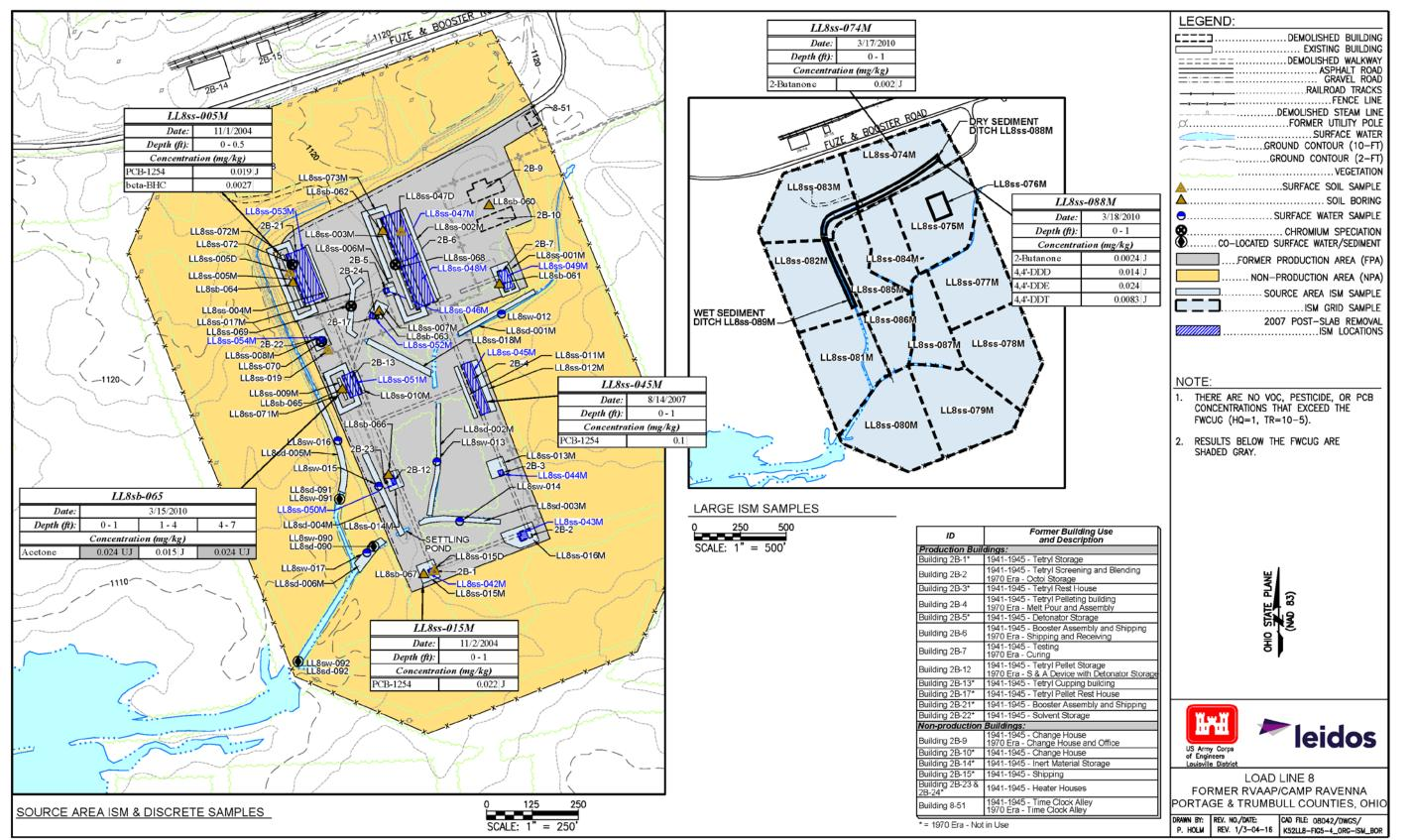
Figure 5-4. Detected Concentrations of VOCs, Pesticides, and PCBs in Soil (ISM and Discrete Soil Borings)
