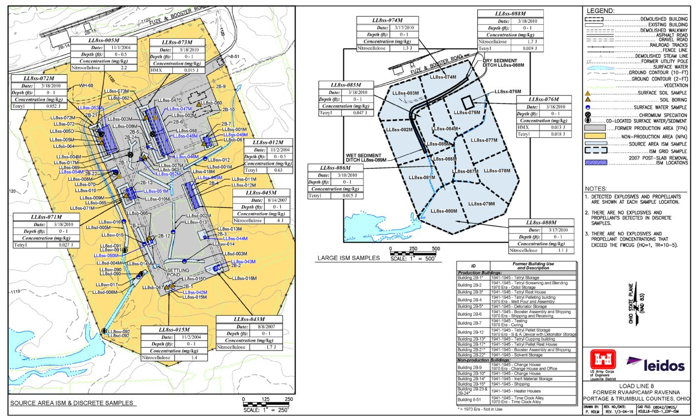
Figure 5-1. Detected Concentrations of Explosives and Propellants in Soil (ISM and Discrete Soil Borings)
