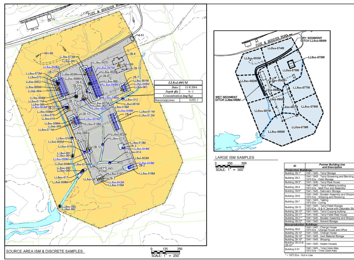
Figure 5-7. PAH Exceedances of FWCUG (HQ of 0.1, TR of 10-6) in Surface Water and Sediment
