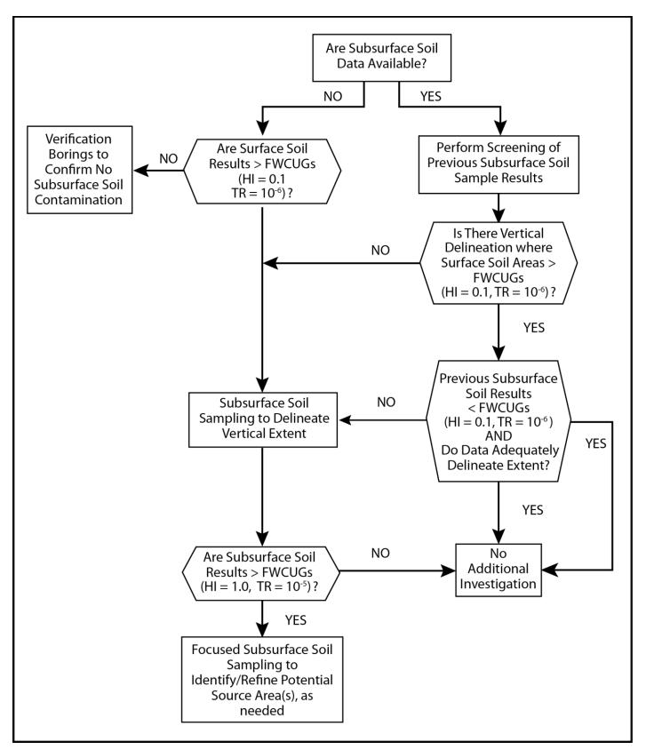
Figure 4-4. PBA08 RI Subsurface Soil Sampling
