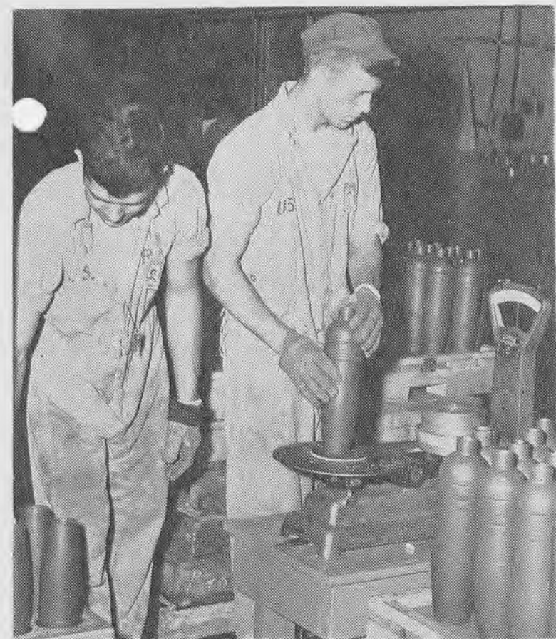
QUALITY CONTROL of Arsenal-loaded 90mm projectiles begins with the above pre-zone weighing operation. Performing this job in Department 66 Line One are H. J. Trivelli of Ravenna and D. R. Swartout of Cuyahoga Falls.
