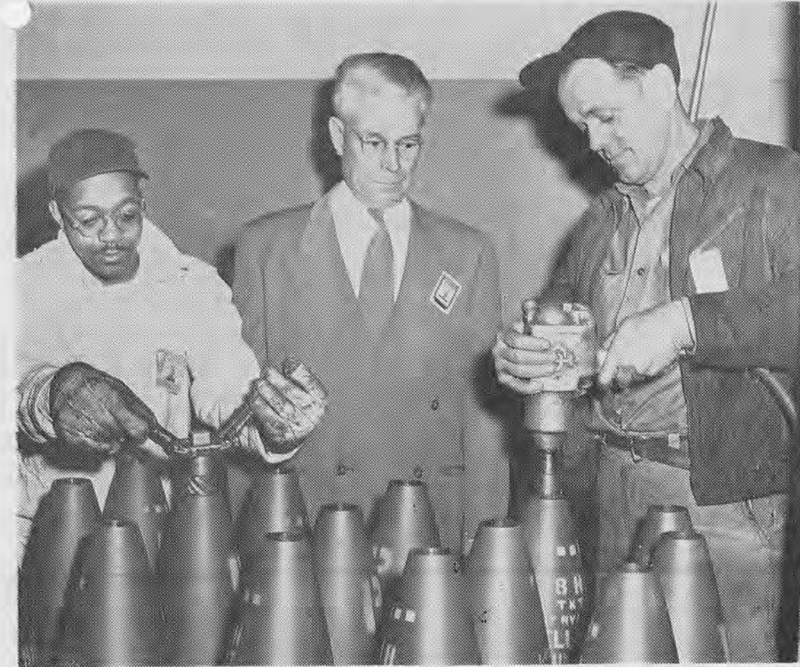
THE OLD and the new way of removing fuze well cups from the noses of 155mm projectiles is demonstrated by Lawrence Steele, Akron, Department 84, and suggestion award winner Raymond C. McDaniels, right. Looking on is H. C. Gantt, Newton Falls, general foreman of Line Maintenance Department.
