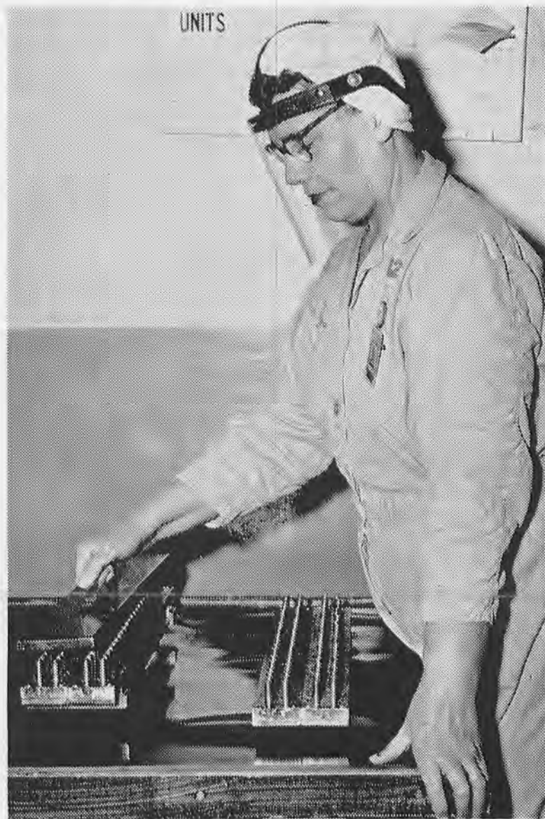
THREE-TIME suggestion award winner, Arla Hoover, demonstrates one of her winning ideas, a primer cover. Mrs. Hoover, who works on the Artillery Primer Line, suggested that a cover be used to prevent the powder shaking out of the primer cases during the vibrating operation. Mrs. Hoover is a Ravenna resident.
