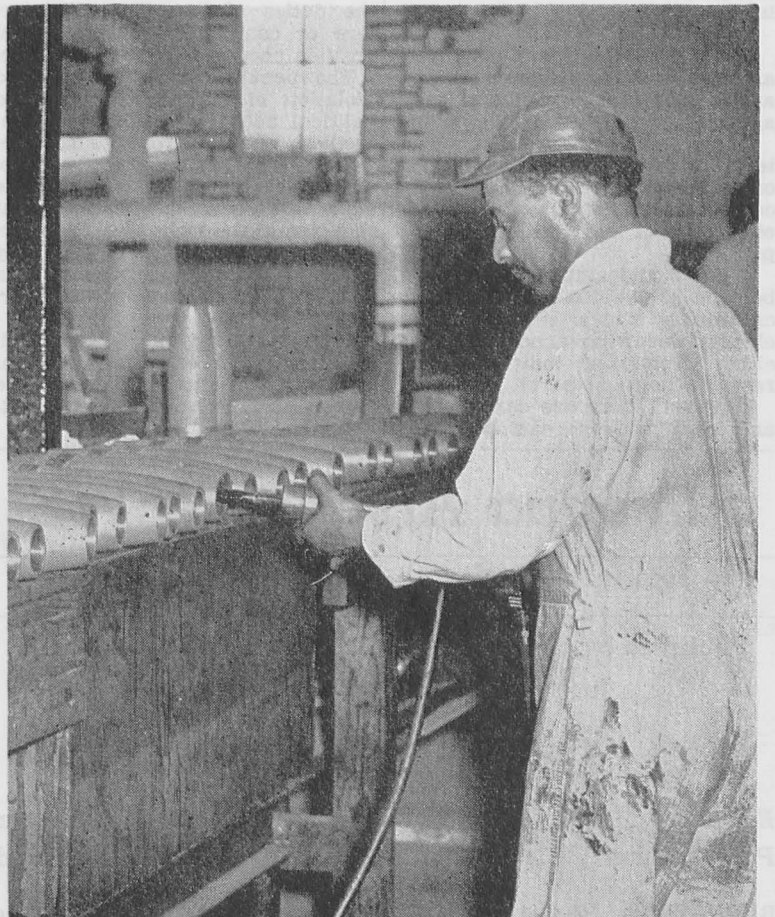
FOR PROTECTION against corrosion, the insides of the clean shells are painted by Henry Williams (above) of Youngstown. After being inspected, the shells are loaded on pallets and shipped to a components magazine. From there they go to the load lines to be loaded with explosives.
