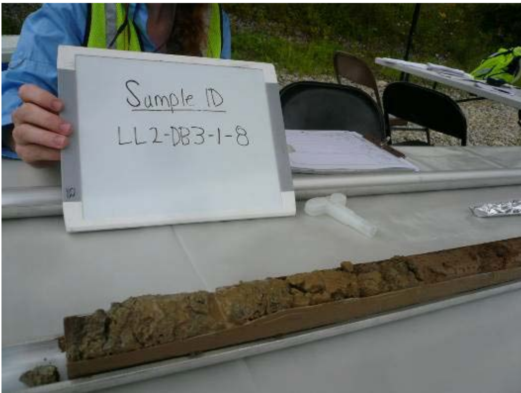
Photograph 4-19: Wet gravel fill recovered at some locations
