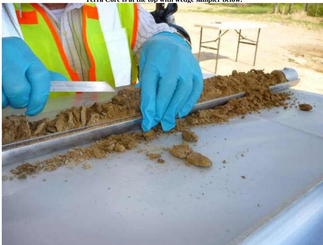
Photograph 4-29: Use of aluminum wedge sampler with weathered rock
