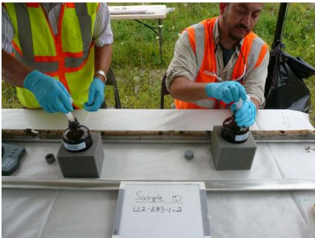
Photograph 4-25 B: Putting nominal 5-gram soil plugs in bottles with Methanol (horizontal subsurface ISM samples)
