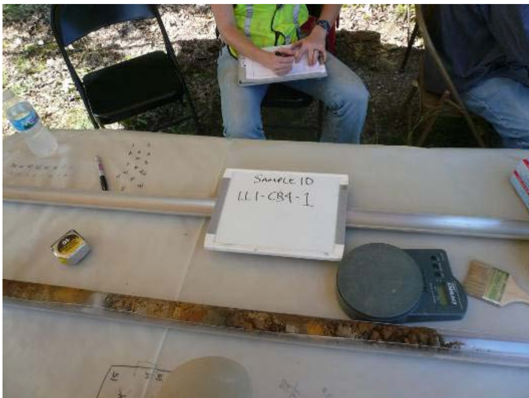
Photograph 4-21: Recent fill over older fill over weathered rock
