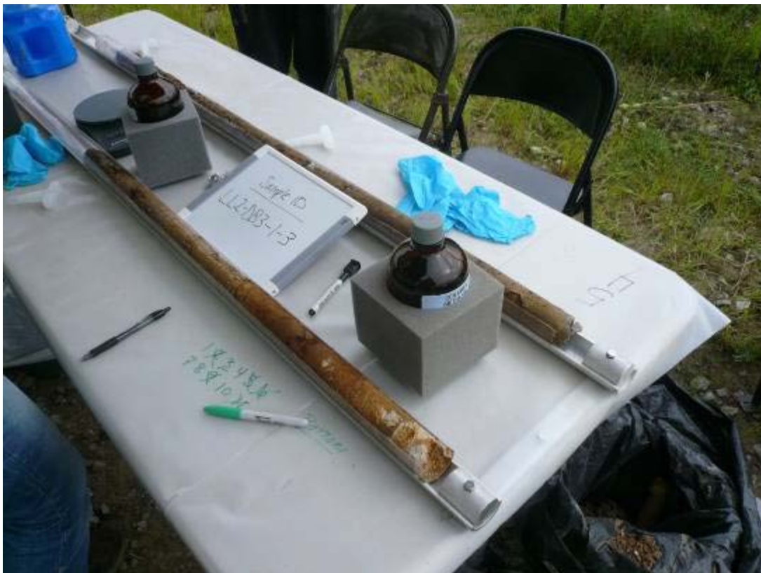
Photograph 4-16: Aluminum half pipes securing Geoprobe tube liner
