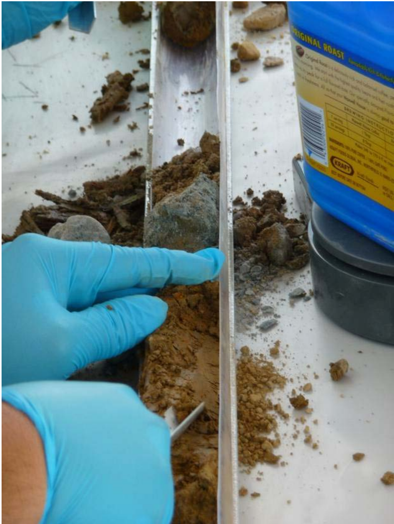
Photograph 4-30: Use of aluminum wedge sampler with hard clays
