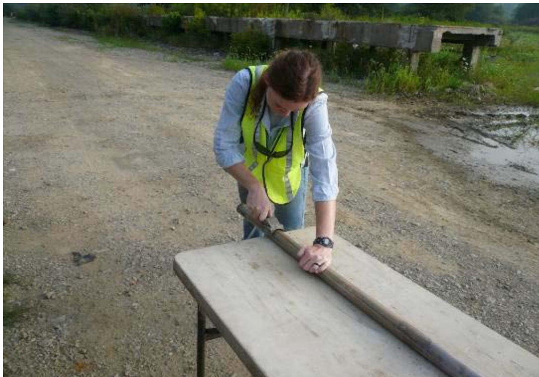
Photograph 4-14: Geoprobe liner cutting
