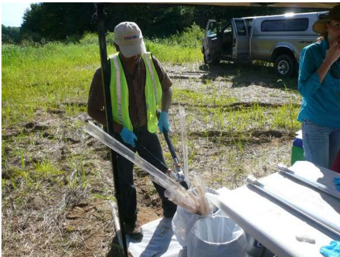
Photograph 7-2: Cutting used Geoprobe liner tubes for easier handling and disposal
