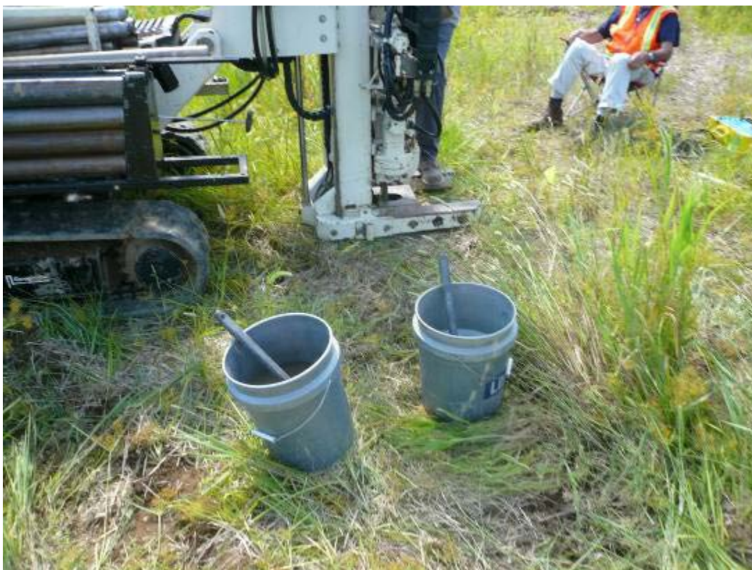
Photograph 4-10: Decontamination of the core barrel shoe.
