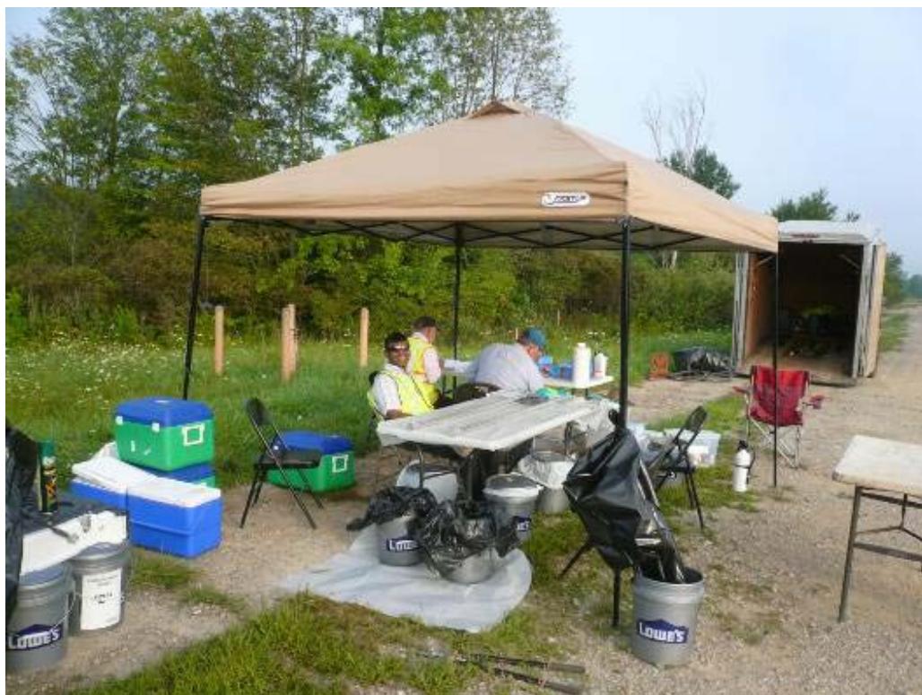
Photograph 4-27: Lined 5-gallon buckets used to collect horizontal subsurface ISM samples. The 3 buckets with white garbage disposal bags are used for the three depth intervals- 1 to 3 feet, 3 to 5 feet, and 5 to 7 feet.
