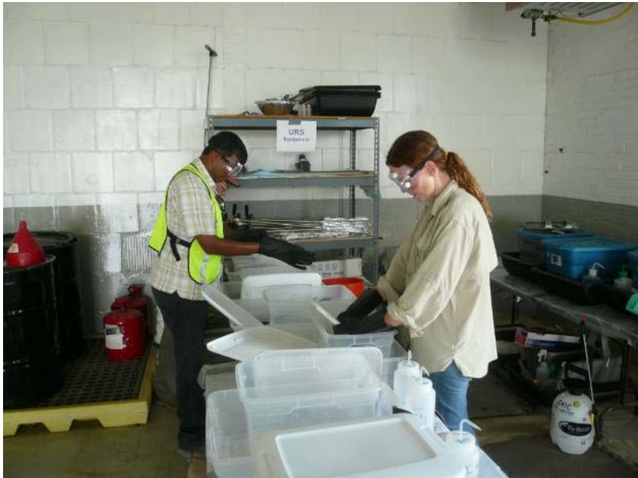
Photograph 6-2: Decontaminating aluminum wedge samplers
