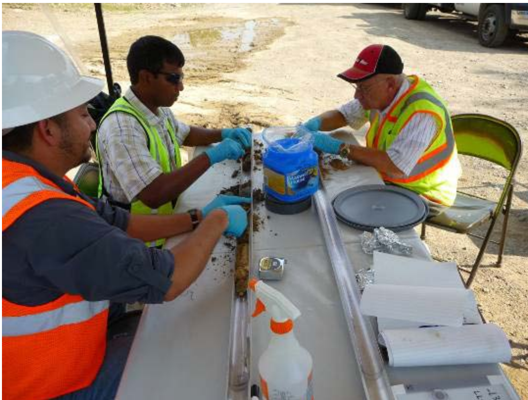
Photograph 4-31: Use of a lined coffee can to collect vertical subsurface ISM samples.
