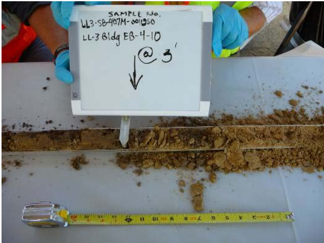
Photograph 4-20: Clay fill over weathered rock
