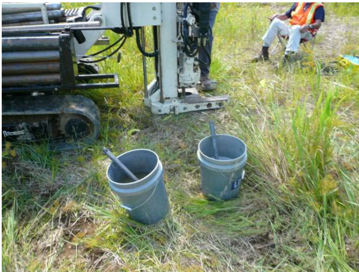
Photograph 6-1: Buckets for field decontamination of the core barrel shoe.
