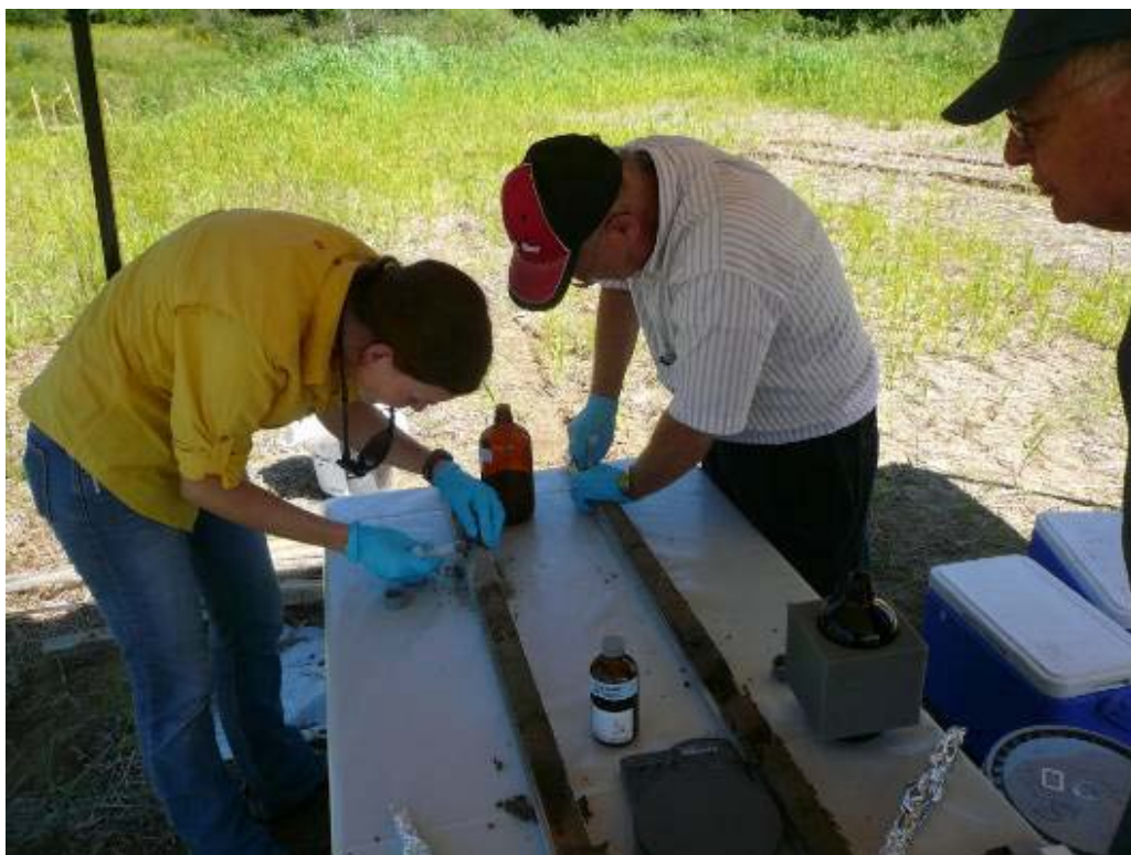
Photograph 4-24 A: Collecting nominal 5-gram soil plugs from the Geoprobe samples. For horizontal subsurface VOC ISM samples, the large, opened jars are used.
