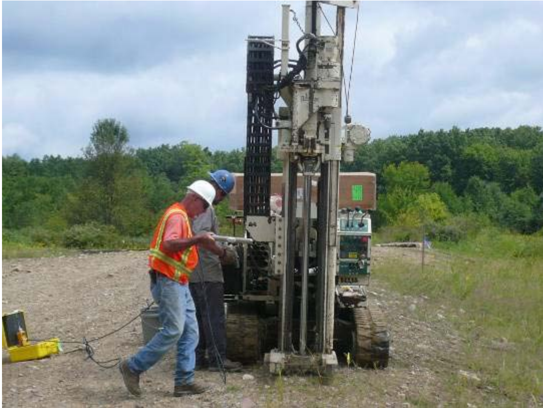
Photograph 4-7: Subsurface anomaly avoidance with Gradiometer Model BHG
