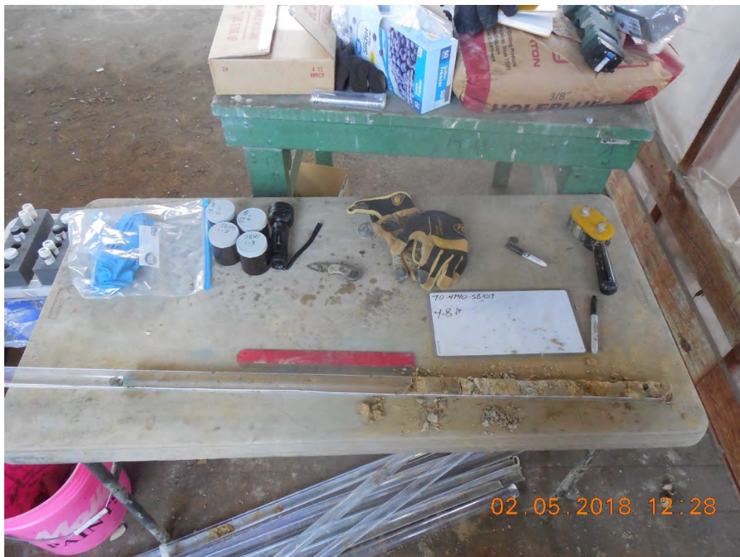
175 Photo 49 (2018): Soil core (4-8 feet) from boring SB107 located adjacent to the storm drain on the 176 southeast corner of Building 47-40 Round House. SB107 is associated with the Outdoor Wash Rack Area 177 (DU06).
