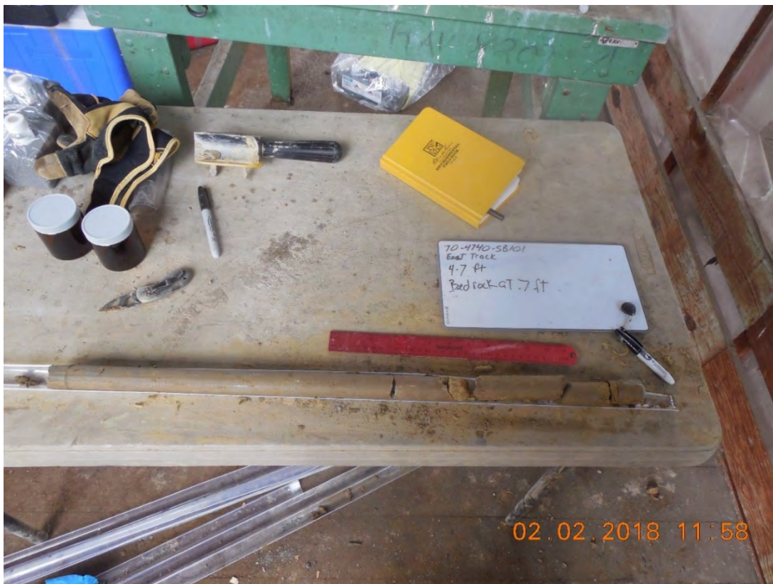
146 Photo 40 (2018): Soil core (4-7 feet) from boring SB101 near the East track where the concrete and wood 147 floors meet within Building 47-40 Round House Interior (DU04).
