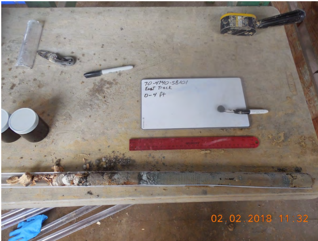
143 Photo 39 (2018): Soil core (0-4 feet) from boring SB101 near the East track where the concrete and wood 144 floors meet within Building 47-40 Round House Interior (DU04).
