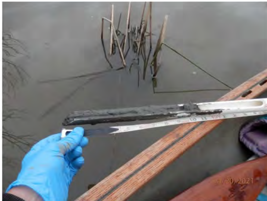
10. Photograph of Depth of sediment at sampling location 079SD-412 located on the East end of the North Transect
