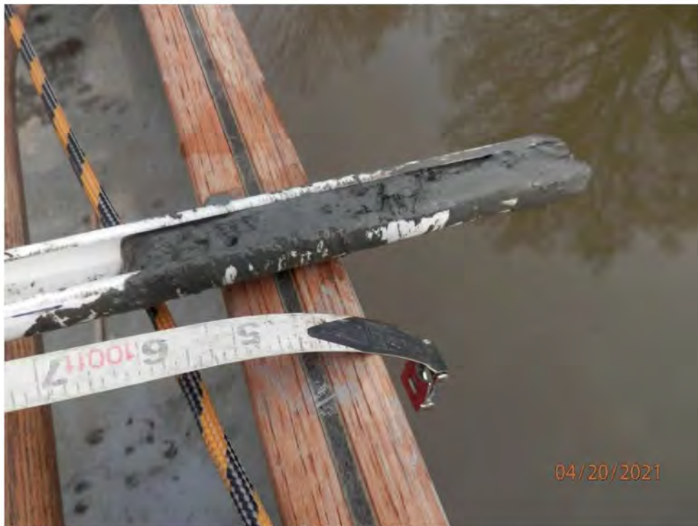
6. Photograph of depth of sediment at sampling location 079SD-411 located from the middle of the North Transect
