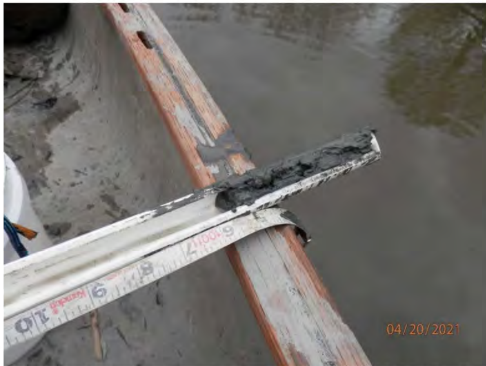
16. Photograph of Depth of sediment at sampling location 079SD-414 located in the middle of the South Transect
