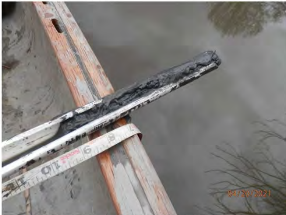
18. Photograph of Depth of sediment at sampling location 079SD-415 located on the East end of the South Transect
