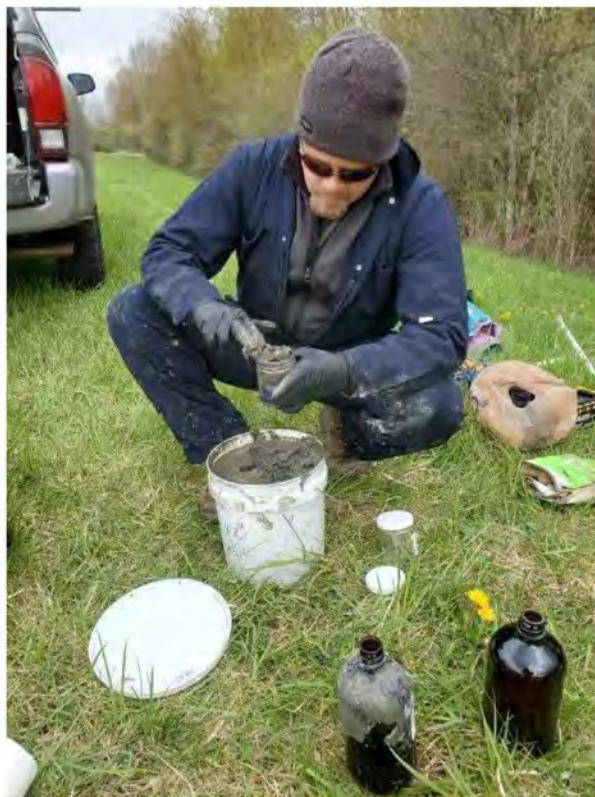
19. Photograph of filling sample jars with collected sediment.
