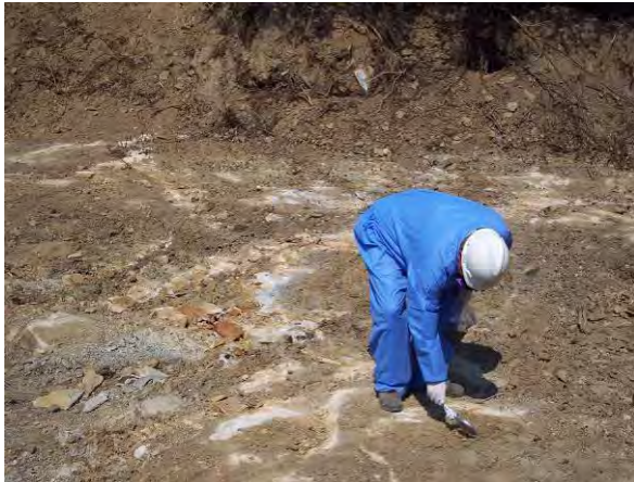
Photograph 3-9. Soil Sampling After Excavation of Removal Area Containing ACM
