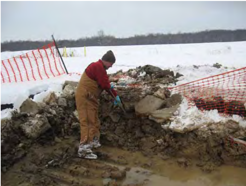
Collecting aliquots of the excavation floor and sidewalls during MI sampling operations.
