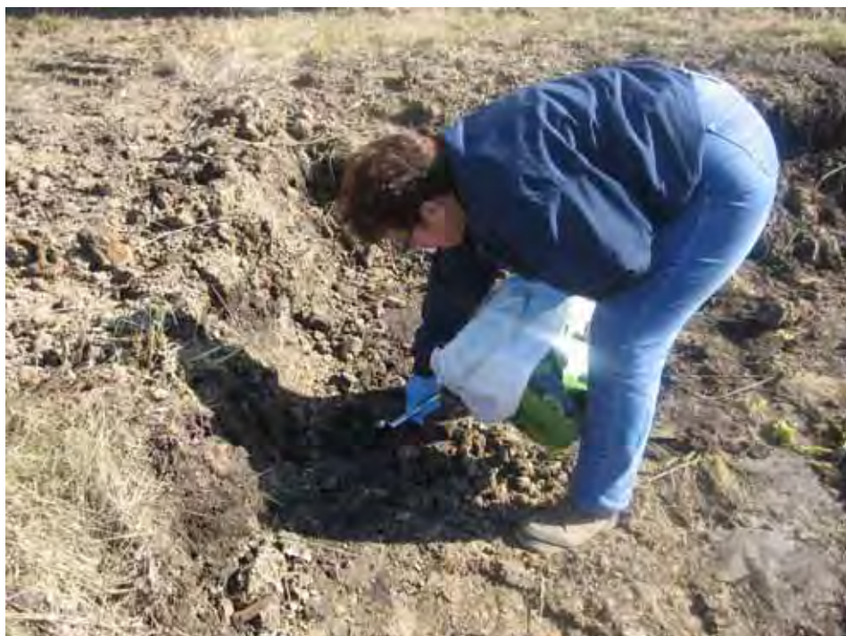
Collecting MI aliquot from floor of excavation at Pad 67.
