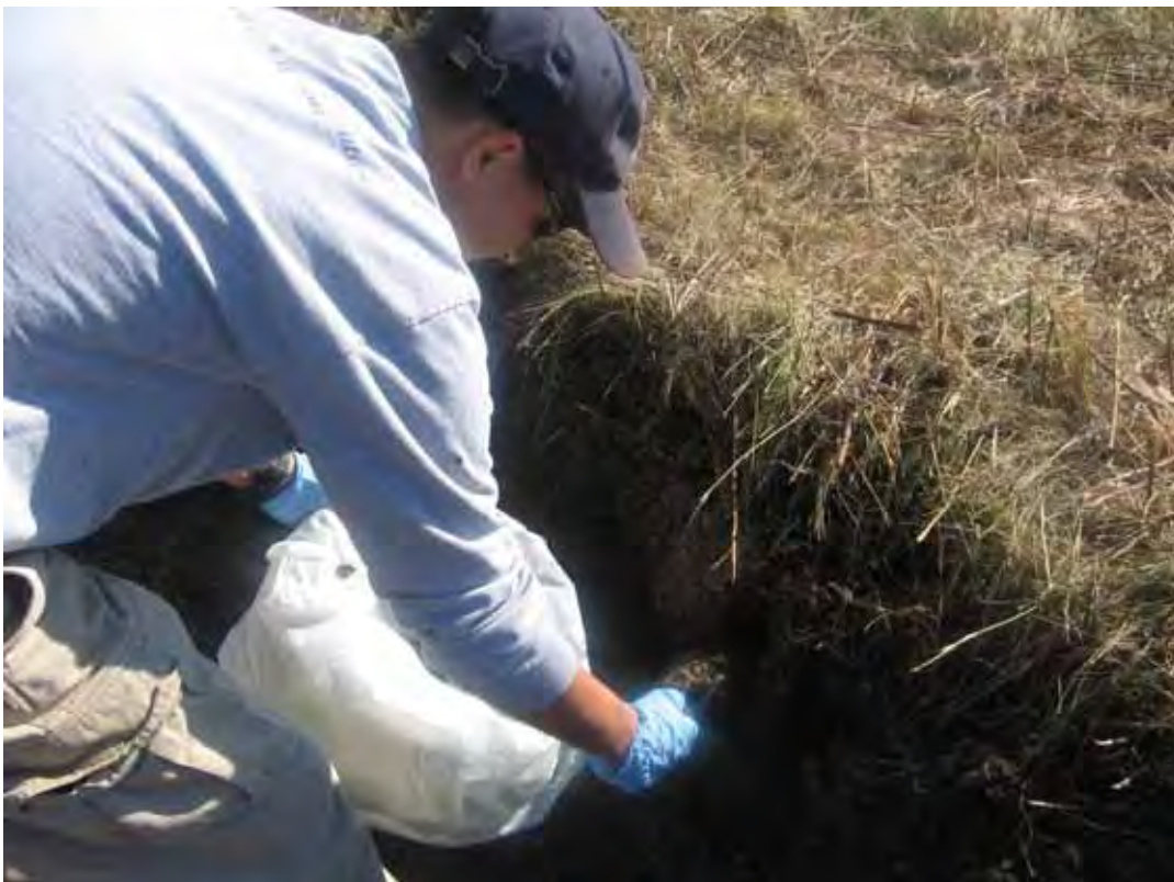
Collecting MI aliquot from sidewall at Pad 67 excavation.
