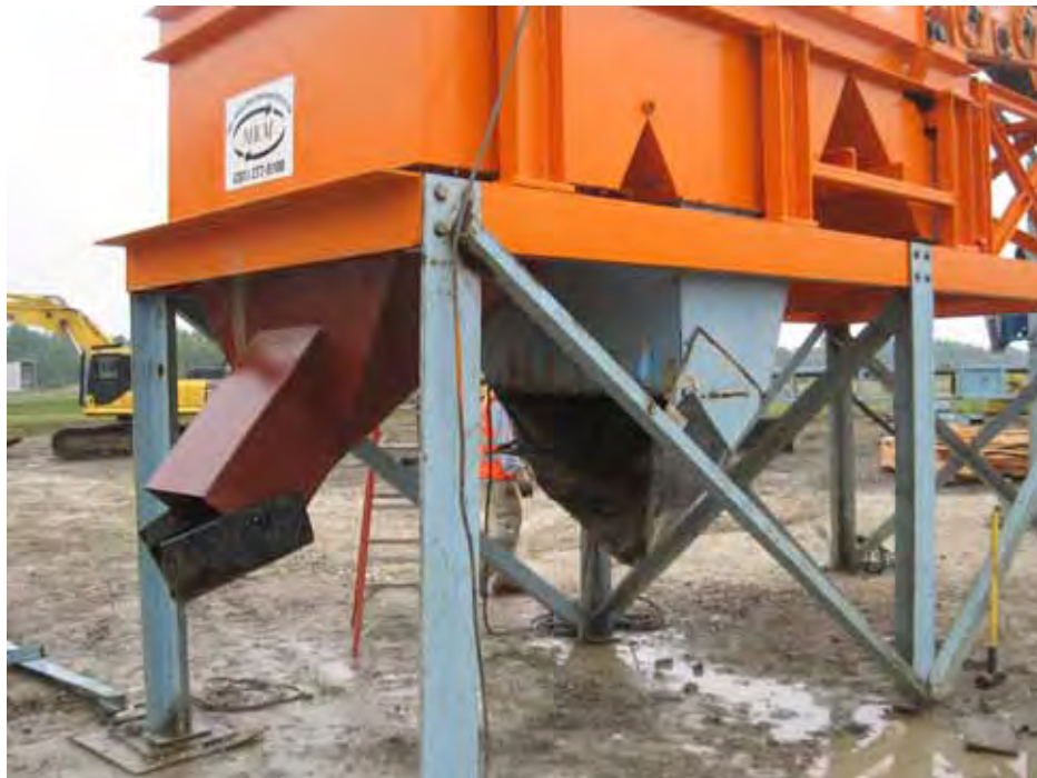
Pictures showing chutes installed on eddy current magnets.
