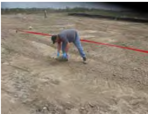
Overview of sample grids established within stockpile footprint to facilitate the sampling operations.
