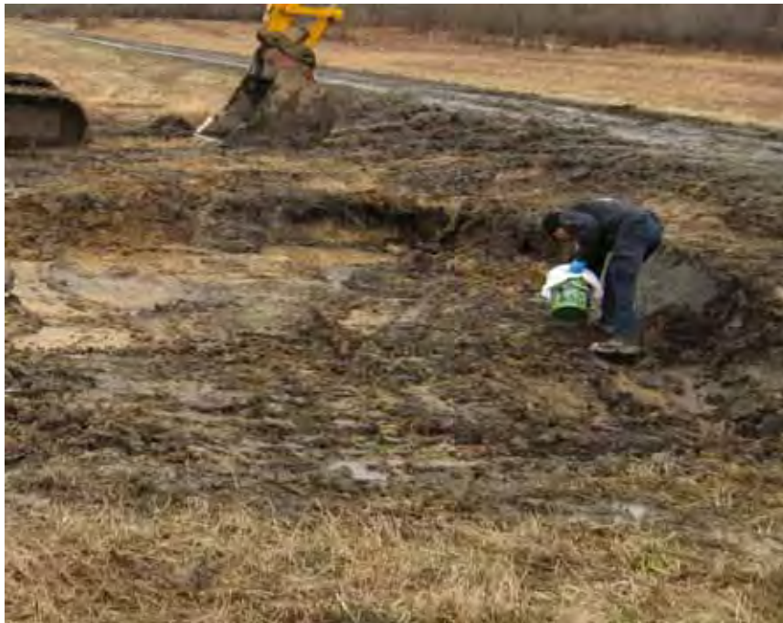
Collecting MI soil confirmation samples from excavation.
