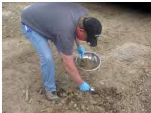
Certified Asbestos Supervisor collecting MI soil sample from within northeast quadrant of stockpile footprint.
