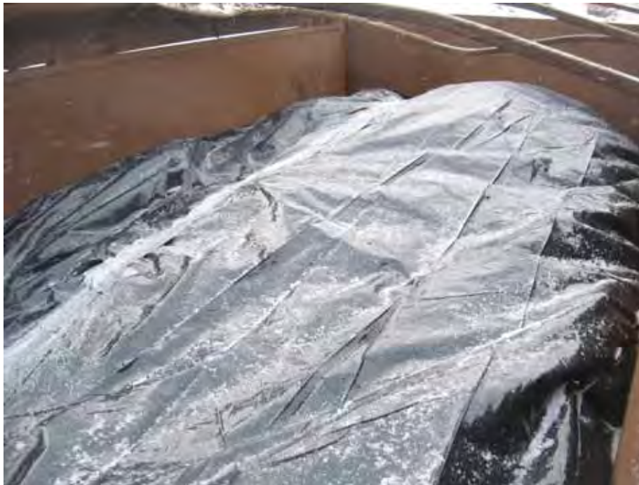
Picture showing liner secured and sealed for transport
