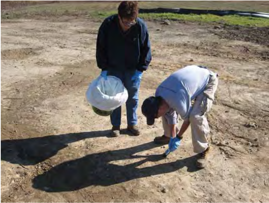
Collecting MI sample aliquot from excavation at Pad 61A (SVOC and RDX).
