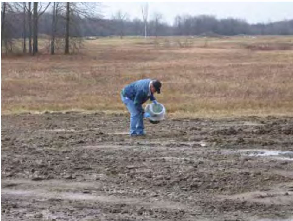
Asbestos supervisor collecting confirmatory asbestos sample at Pad 70 following visual inspection of the area. No ACM noted.
