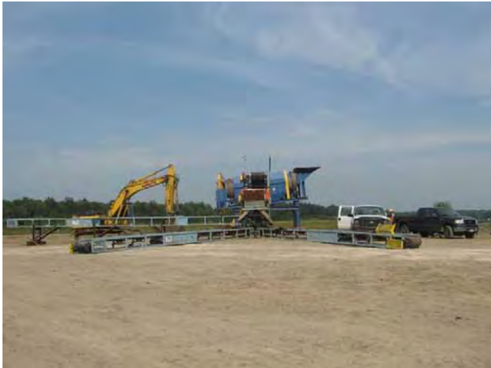
Picture showing set up of the trommel screen and conveyors.
