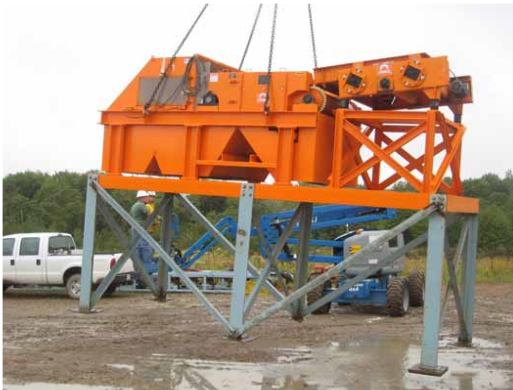
Positioning eddy current magnet during setup.
