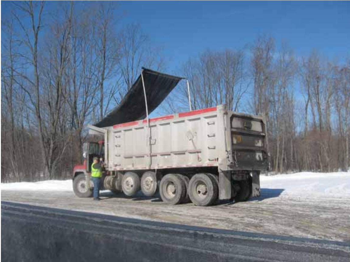
Installing travel tarp prior to exiting site.
