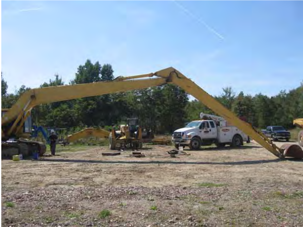
Picture showing long boom installed on excavator. Long boom is needed to provide reach for loading trommel screen.
