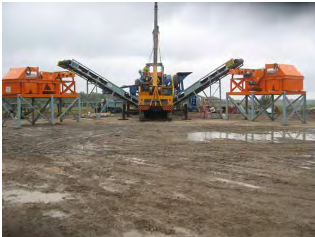
Picture showing both eddy current magnets in place.
