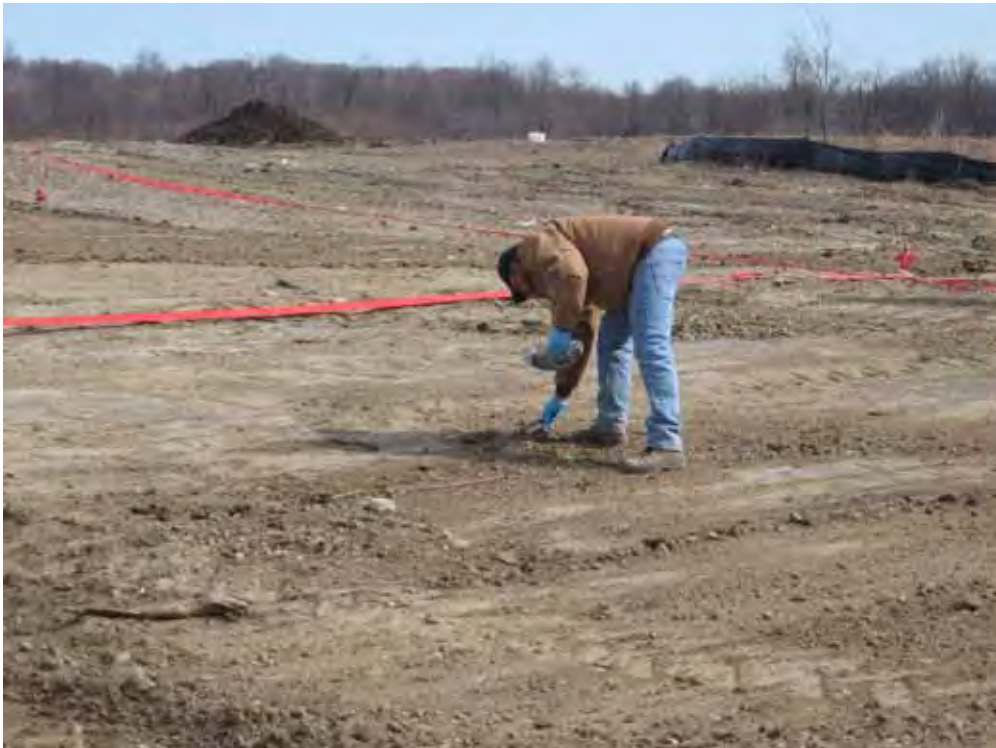
Collecting resample with stockpile footprint.
