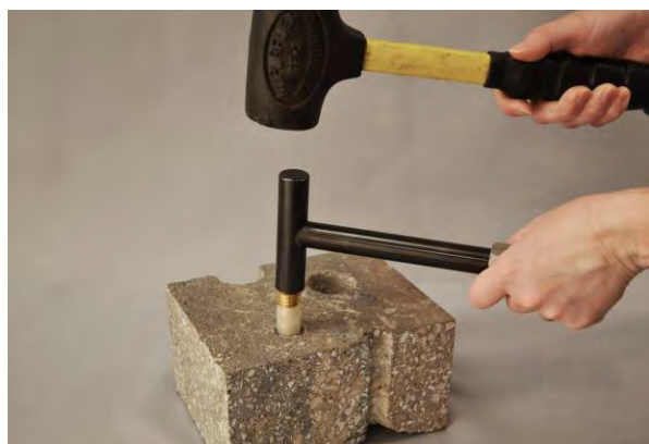
Figure 2. Installing the Vapor Pin™.
