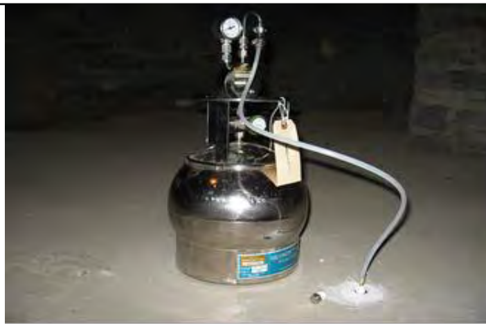
Figure 2: Swagelok® port connected to canister and ready for sampling
