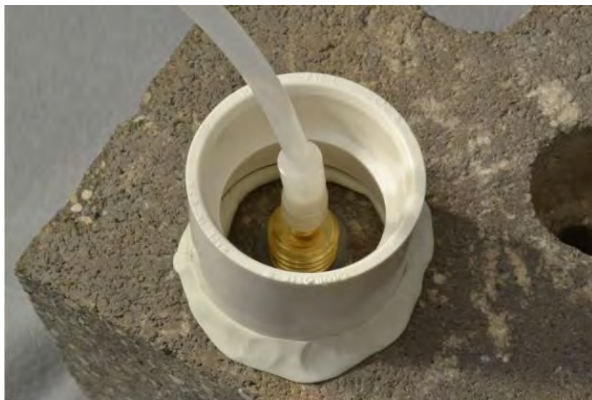
Figure 6. Water dam used for leak detection
