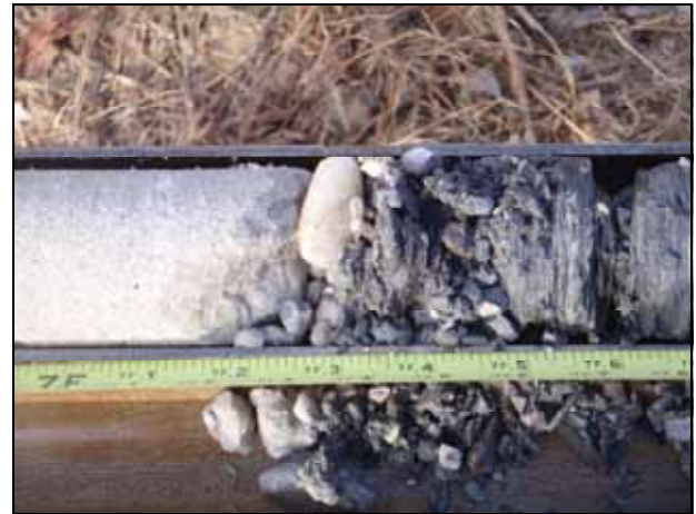
Photograph 2-8. Sharon Conglomerate and Cuyahoga Formation Unconformity
