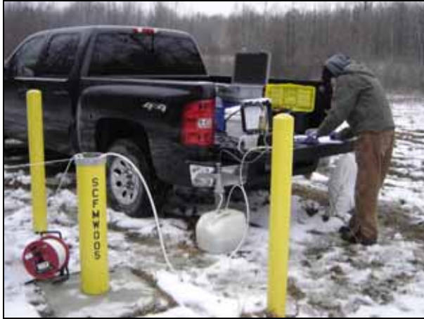
Photograph 2-11. Collection of Water Quality Parameters during Monitoring Well Purging
