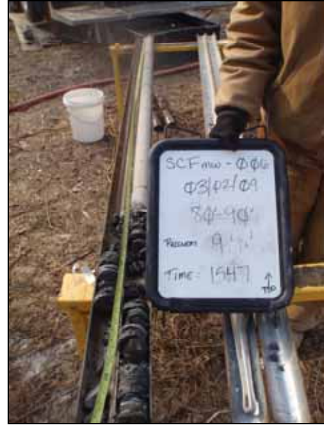
Photograph 2-6. Recovered Section of Rock Core at SCFmw-006
