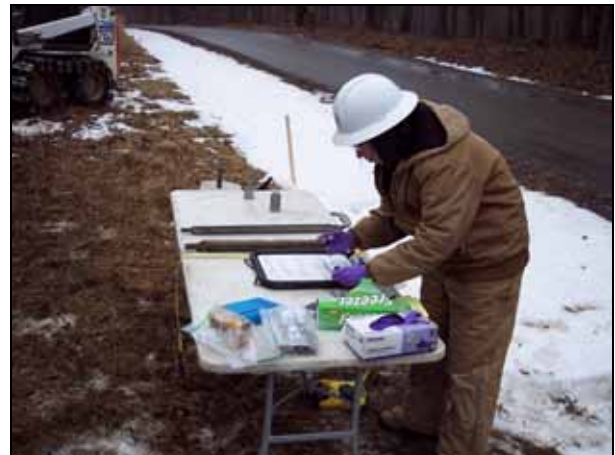
Photograph 2-2. Collection and Description of Soil Samples Obtained with Split Spoons
