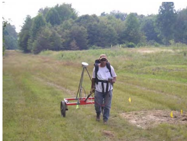
Figure 2-1: EM61 MK2 and Operator
