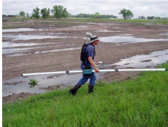
Figure 2-2: EM31 MK2 and Operator
