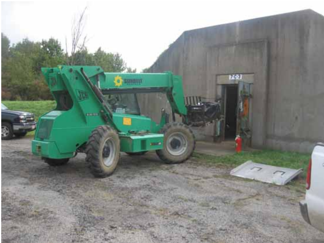
Removing container of 152 mm tracer elements for inspection.
