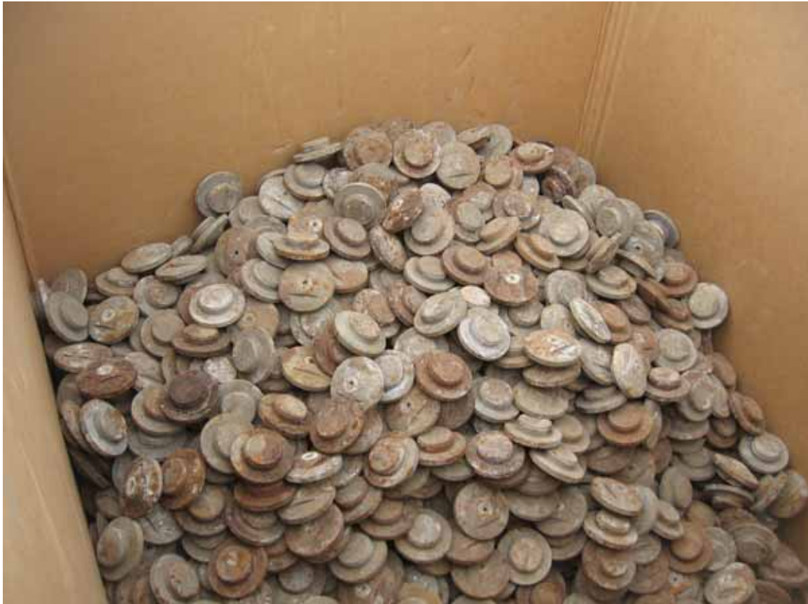
New box filled with inspected 152 mm projectile tracer elements categorized as Material Documented as an Explosive Hazard (MDEH). This material to be stored in ECM 7-C-3 and will require thermal flashing for "Safe" certification under separate contract.
