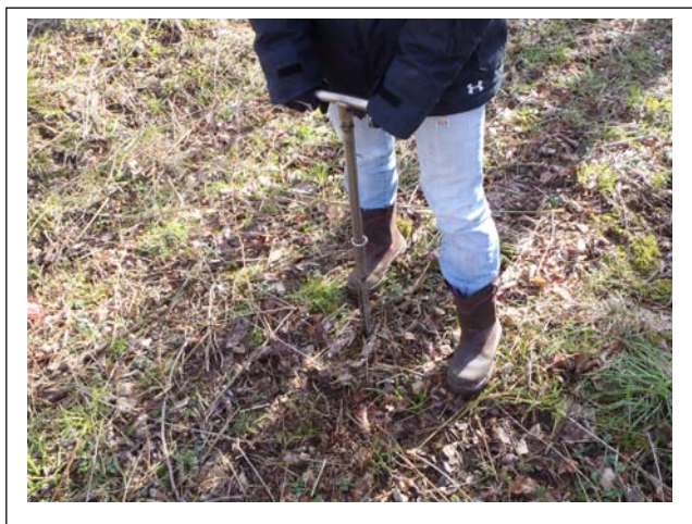
ISM Surface Soil Sample Dedicated Stainless Steel Push Probe
