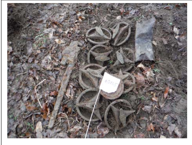
Example of comingled propellant tops and metallic debris
