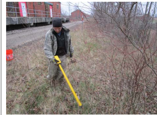
Magnetometer Assisted Anomaly Reacquisition
