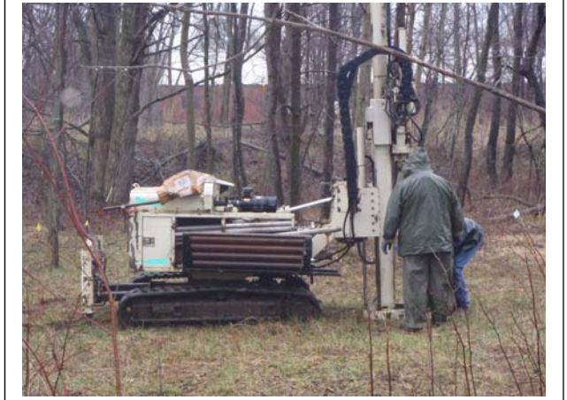
Track-Mounted Geoprobe Drilling – Direct Push ISM Shallow Sub-Surface Sampling
