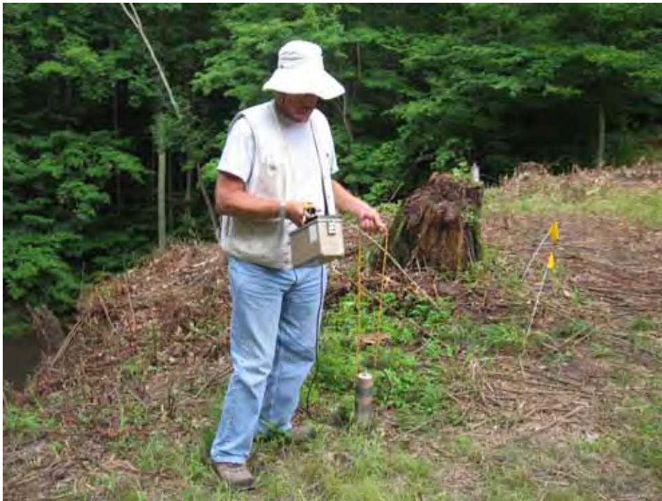
Picture showing Senior Health Physics Technician conducting radiation screening survey along top of slope.
