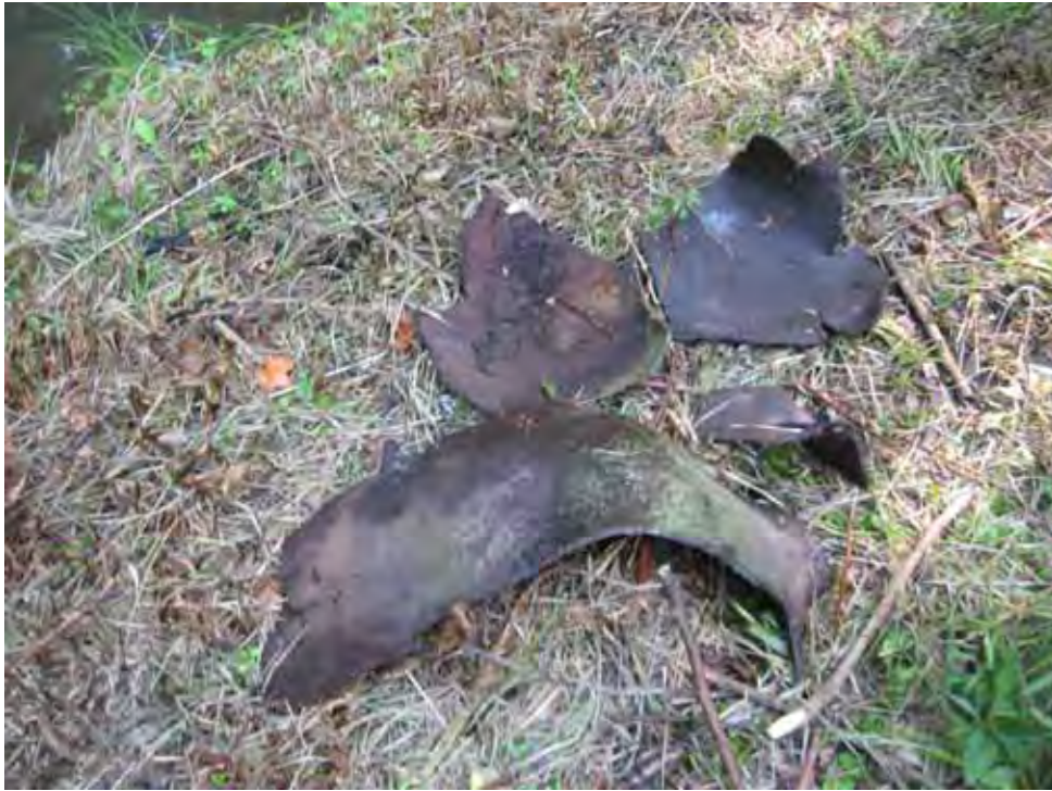
Picture showing all remnants of the third 500 lb bomb that were unearthed and inspected for visible explosive residue.
