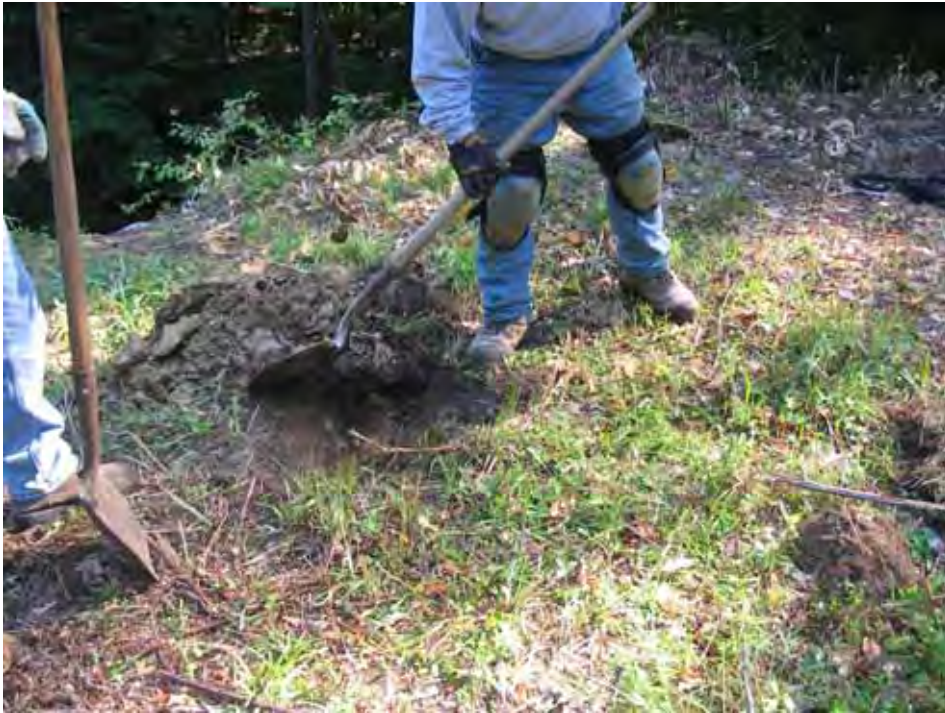
Digging test pit to verify lateral extent of dump area along top of slope.
