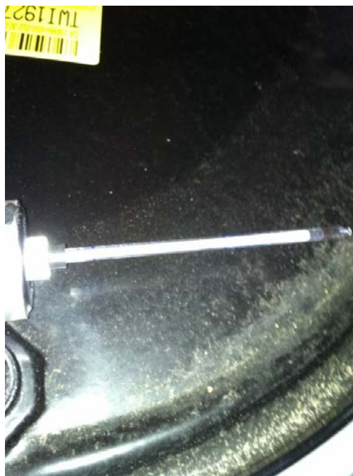
6/14/11 Air monitoring (colorimetric tube) during Load out. Nothing detected on tube.
