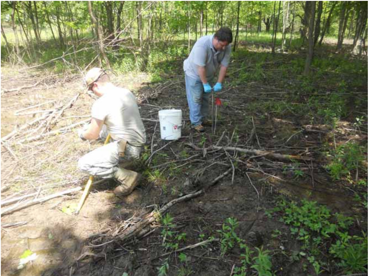
Pictures showing MI surface soil sampling operations with UXO support.
