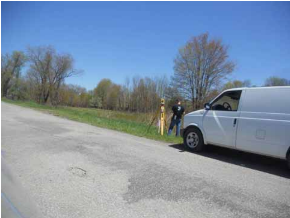
Surveying and installing site grids at Group 2 area to facilitate the geophysical survey.
