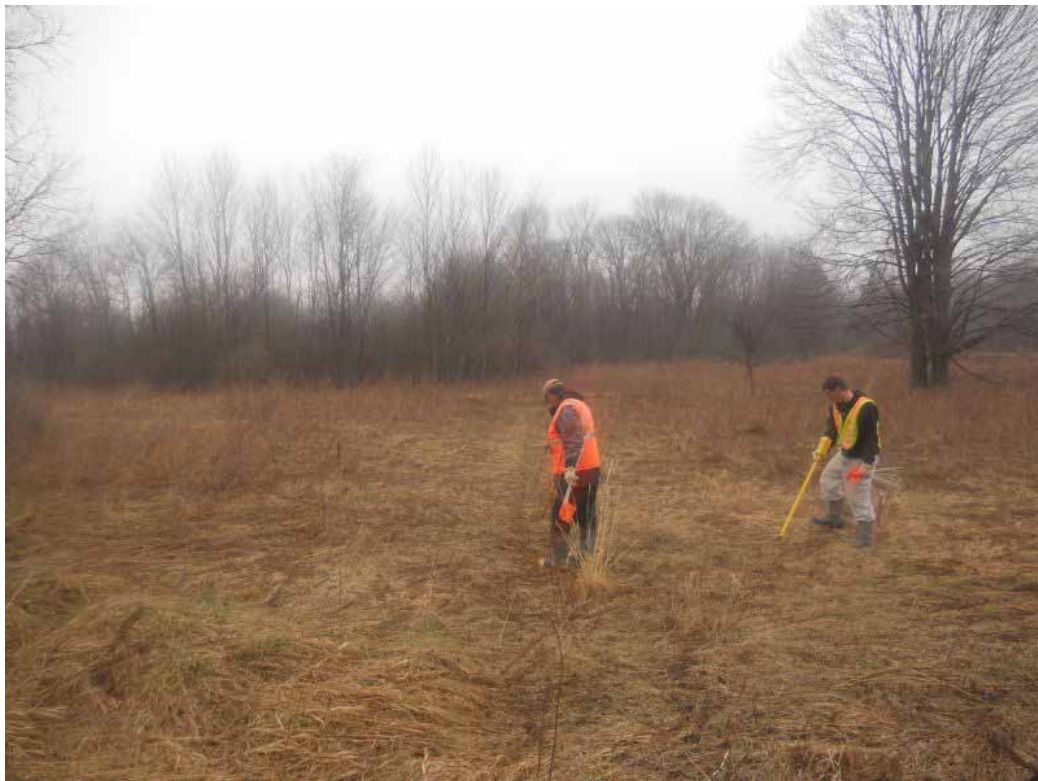
UXO technicians conducting surface sweep operations with Group 2 Propellant Can site.
