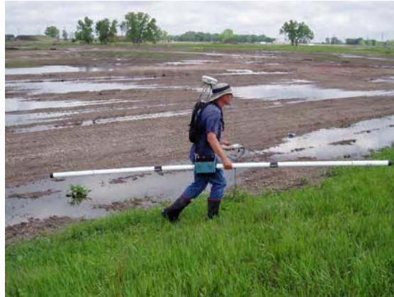
Figure 2-2: EM31 MK2 and Operator
