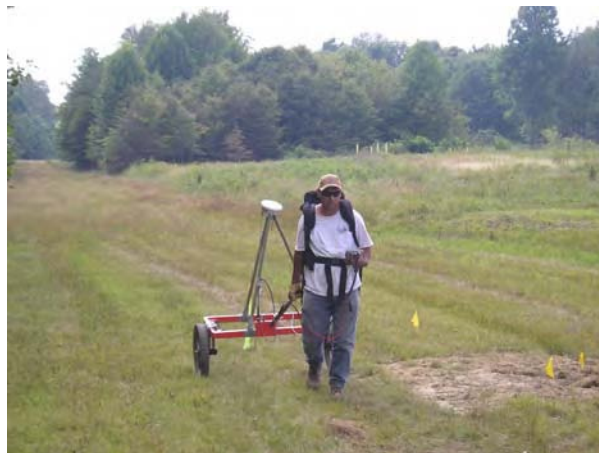
Figure 2-1: EM61 MK2 and Operator
