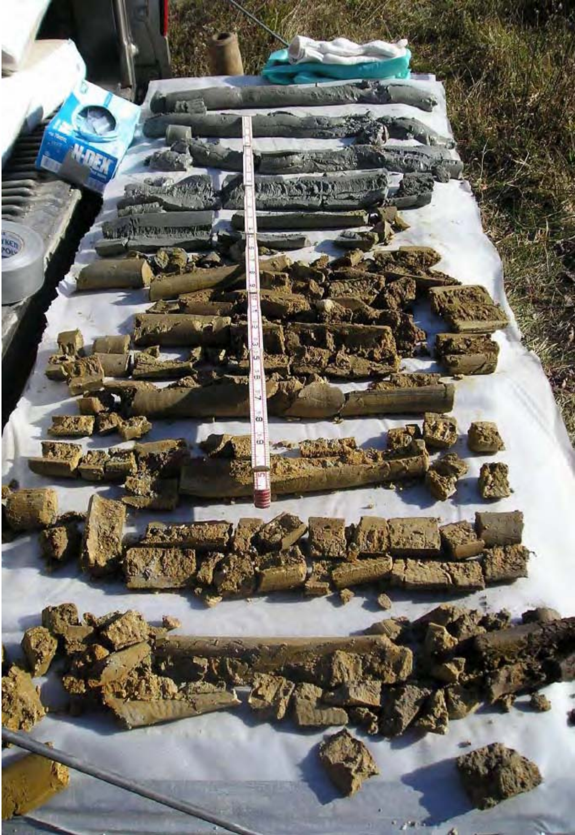
042 - Soil core samples from drilling operations
