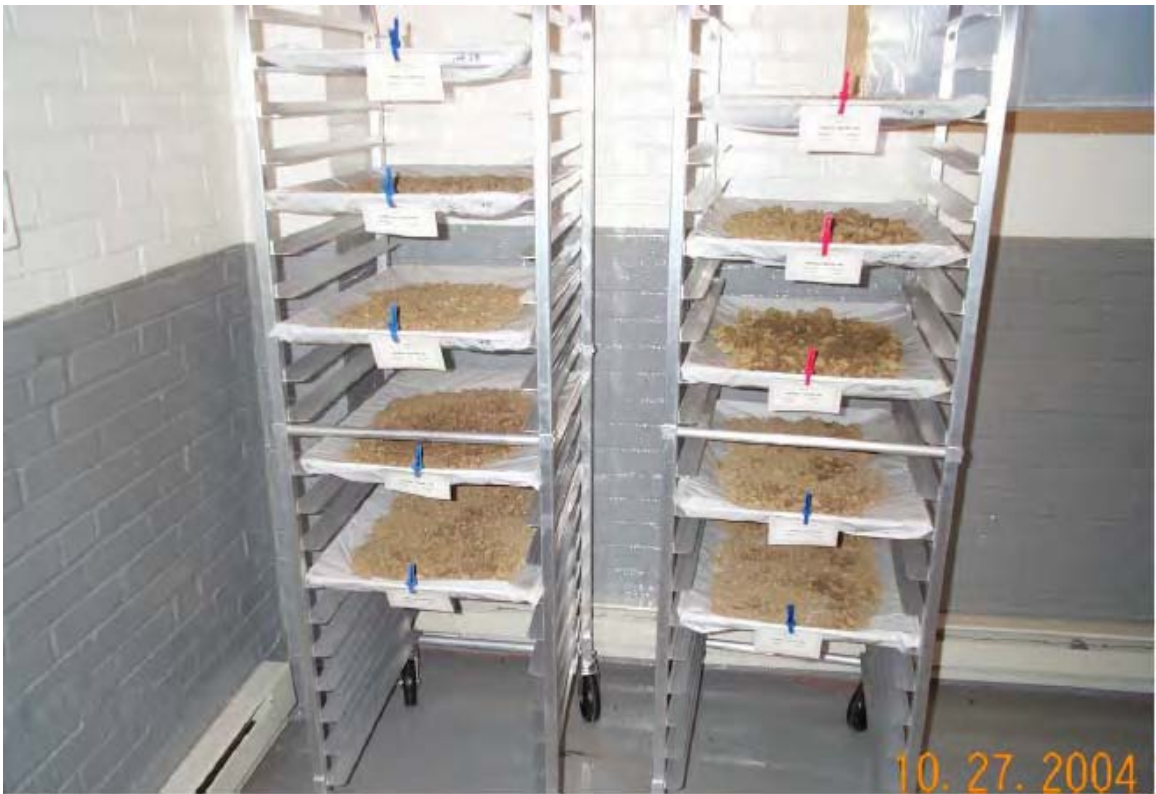
074 - Shallow soil MI samples prepared on drying racks.
