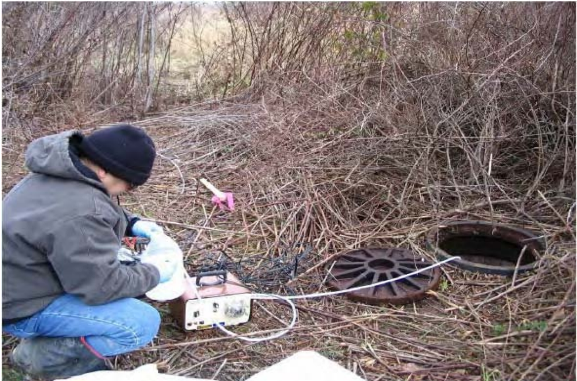
024 - Sewer water collection at LL 7. The sample technician is collecting water to record the water quality parameters.
