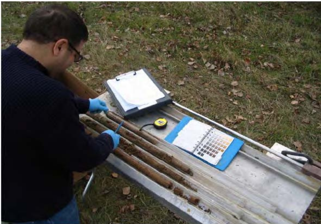
038 - Geologist conducting descriptions of the subsurface soil samples.
