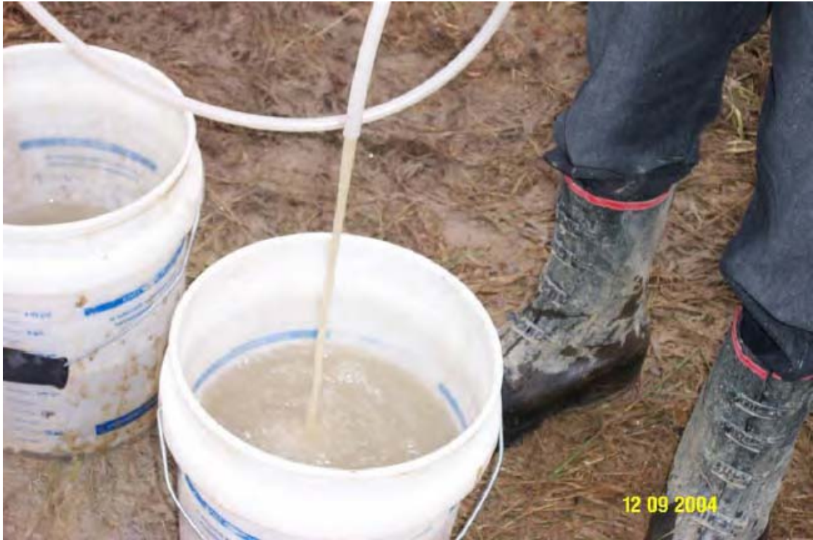
055 - Groundwater monitoring well development at NACA Test Area.
