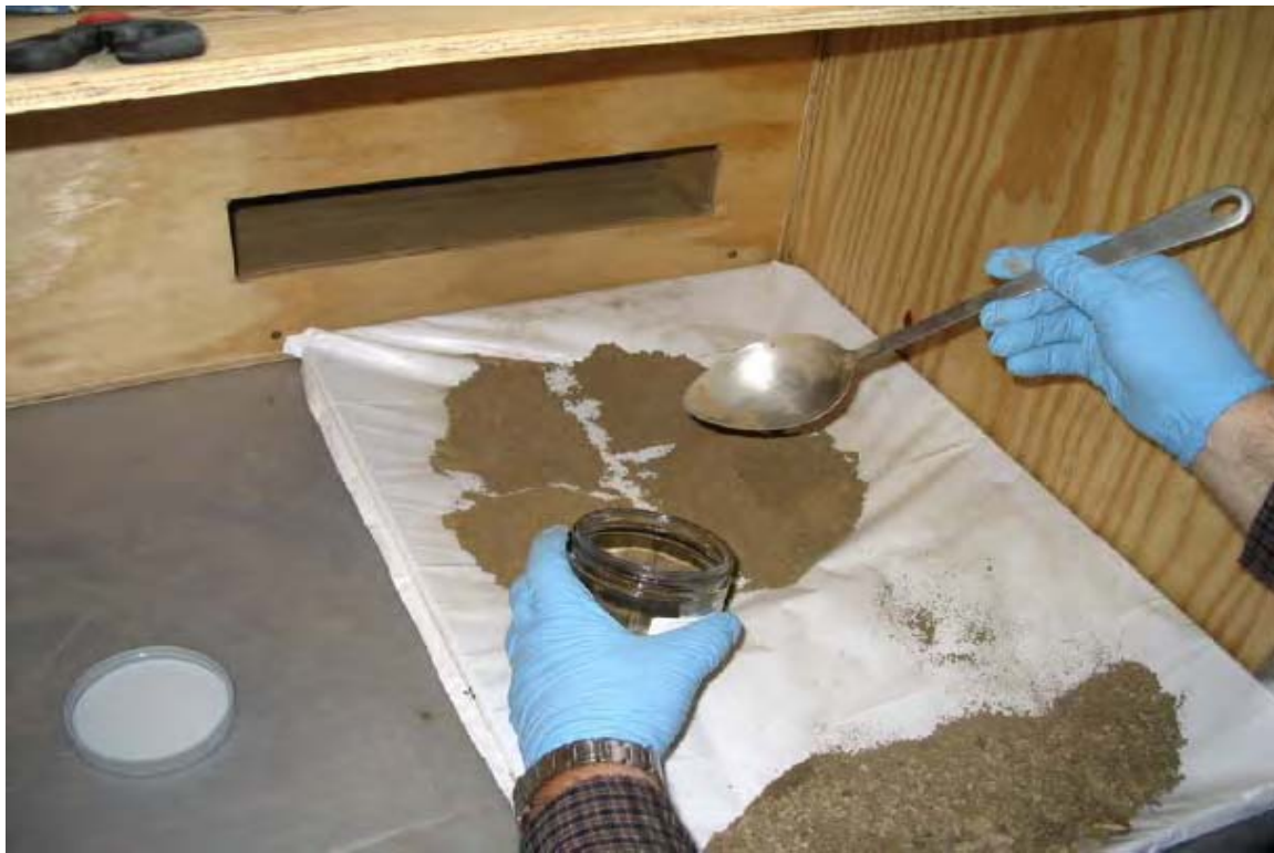
080 - Ground sample material was divided into quadrants and incrementally placed into sample jars.
