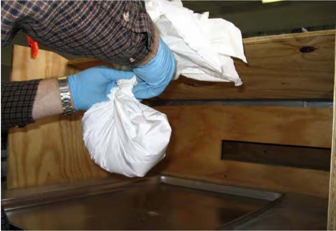
081 - The tray liner is folded in on itself and placed into the IDW disposal container for final disposition at a later time.
