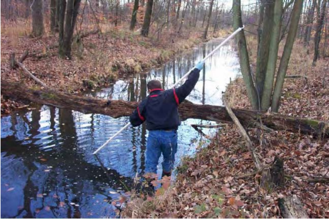
023 - Sediment sample collection at LL 8.
