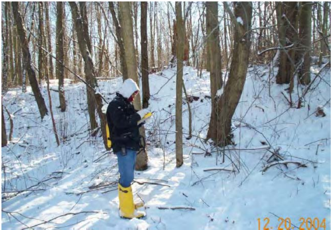
072 - Collecting GPS data from grid corners and discrete sample locations.
