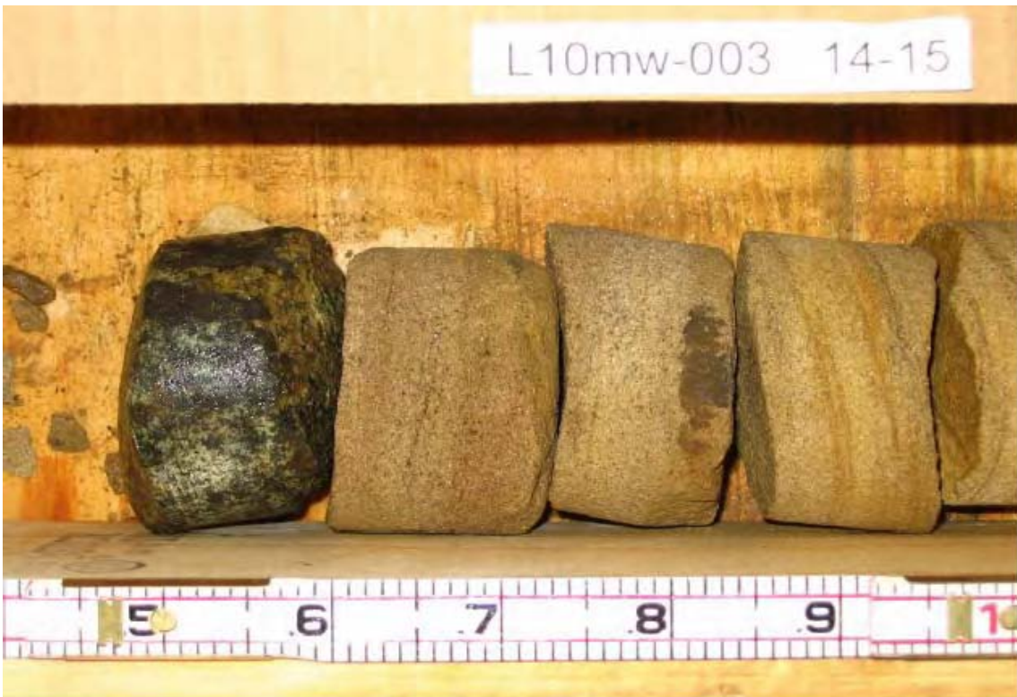
044 - Bedrock core collected from LL 10 (LL10mw-003).
