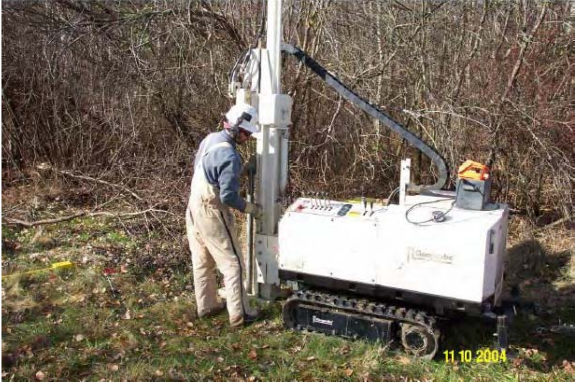
037 - Geoprobe rig and operator collecting a subsurface soil sample at the Landfill N. of Winklepeck.
