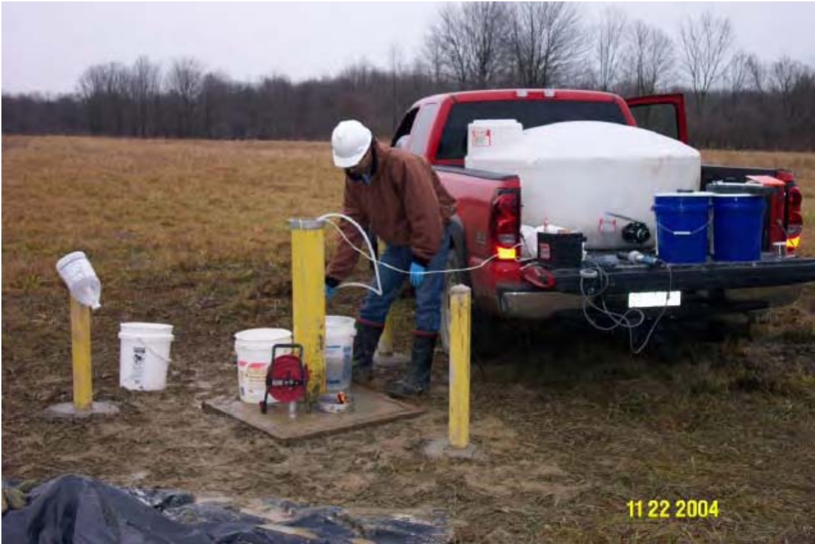
054 - Groundwater monitoring well development at NACA Test Area.
