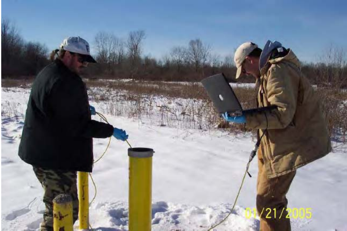
061 - Slug testing of groundwater monitoring wells.
