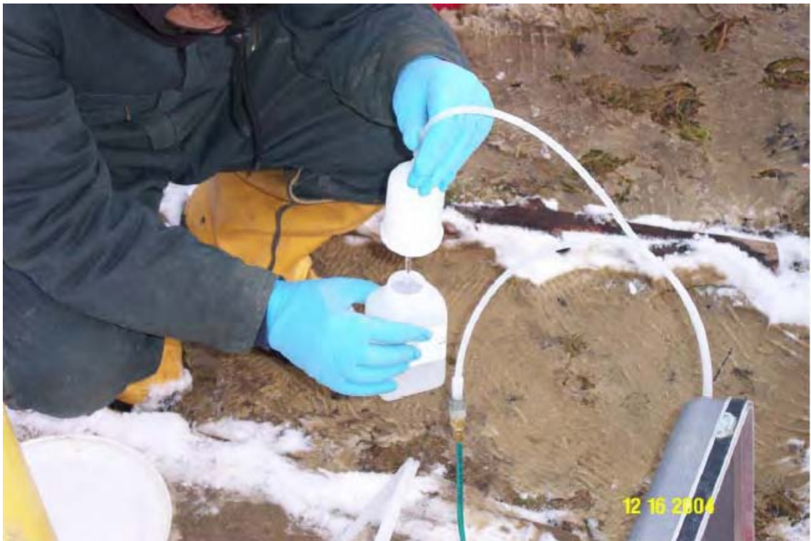
066 - Collection of a filtered groundwater sample for TAL Metals at NACA Test Area.
