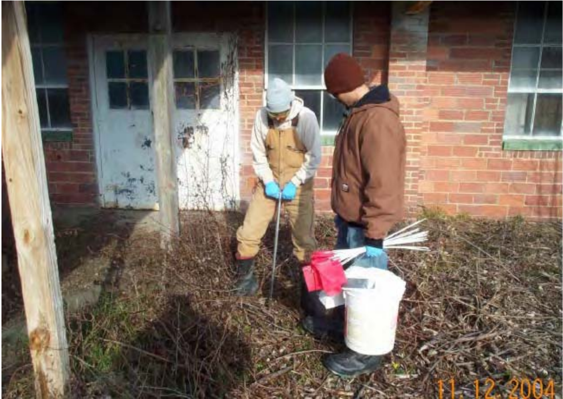
015 - Shallow soil multi-incremental sampling at LL 5.
