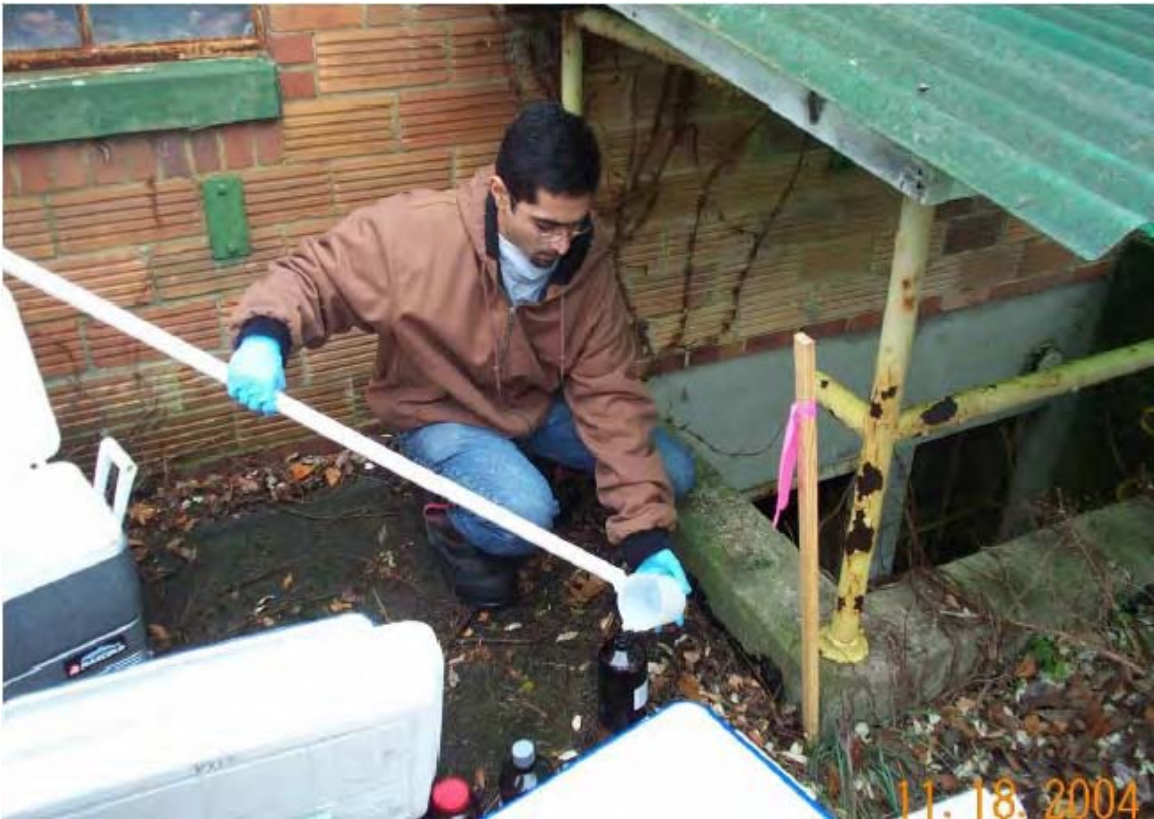
046 - Basement water sampling at LL 5.
