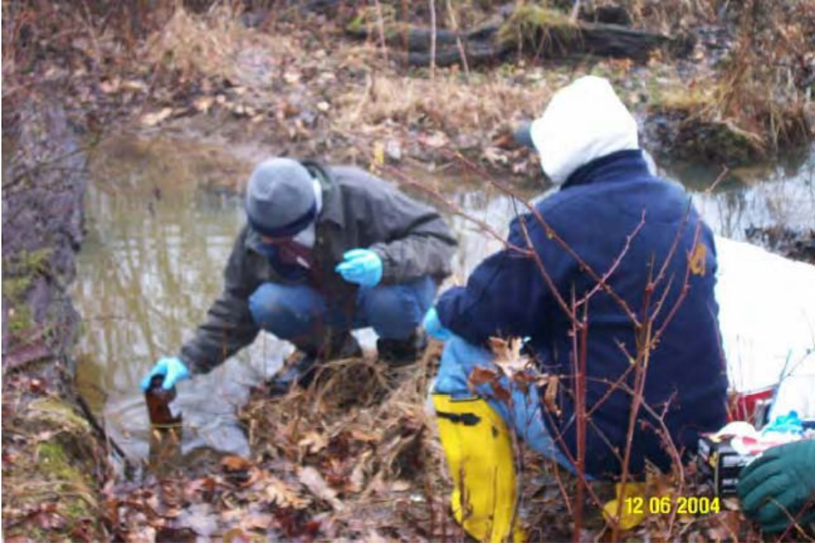
045 - Direct fill surface water sample collection at the Landfill North of Winklepeck.
