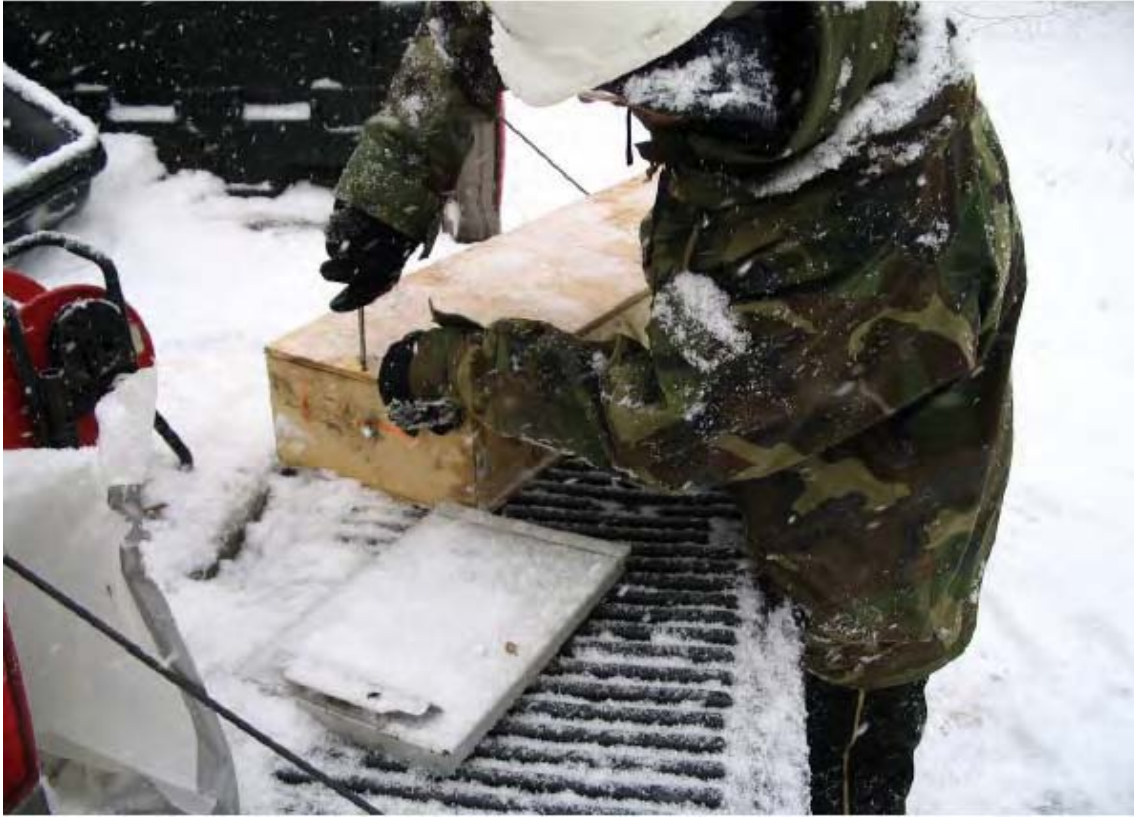
043 - Sealing core sample boxes.
