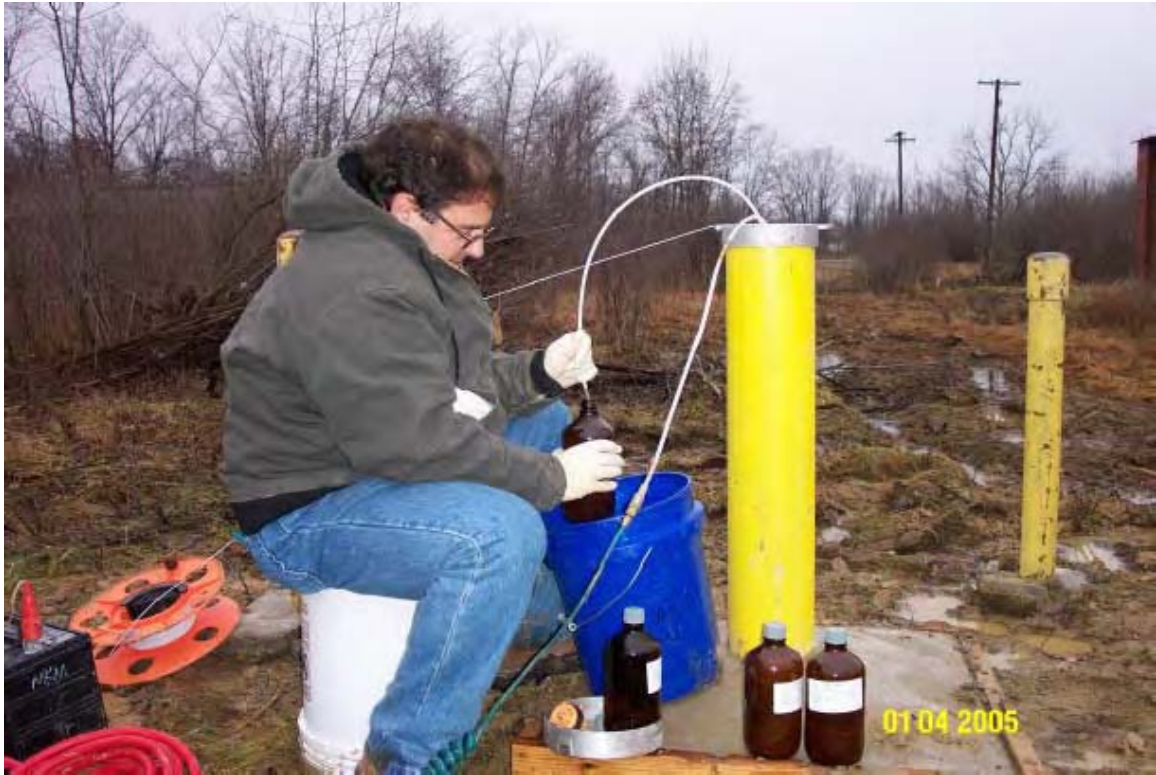
067 - Groundwater sample collection at LL 5.
